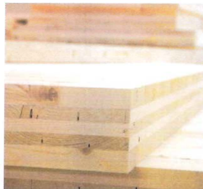
LenoTec elements consist layers of spruce boards bonded crosswise. They are manufactured in sizes of up to 4.8 x 20.0 m – and with thicknesses of max. 30 cm.
