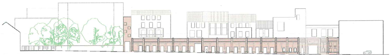
Elevation of the old textile factory wall along Nonnemeersstraat with new openings leading to the covered gallery space beyond.
